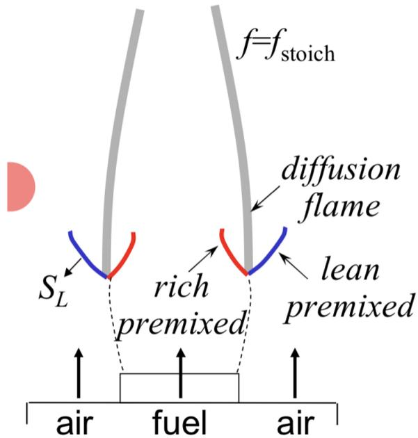
Figure 10: Partially Premixed Combustion
