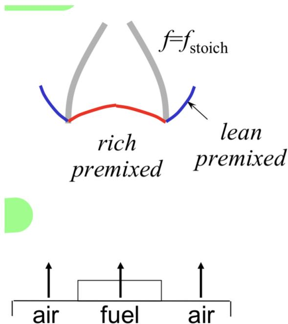
Figure 11: Higher Speed Partially Premixed Combustion
